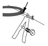
**8.** There should be no space left between the tensioner's head clamp and the ring
