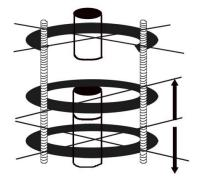
**7.** Apply distraction between the distal and middle rings, acting on the nuts on the middle ring
