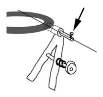
**9.** Tighten the screw on the back of the tensioner
