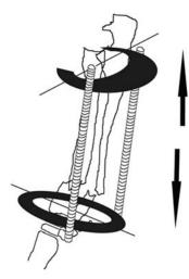
**5.** Distract the fracture acting on the nuts On the threaded bars. If needed, add a third threaded bar for reduction.
