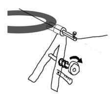
**13.** You can release pressure on the handles when the tensioner is locked, and measure the tension using the conversion chart
