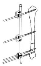
**7.** Lock each clamp to the connecting bar. Complete the stabilization as required by the fracture features.
