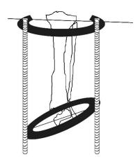
**4.** Connect the rings with threaded bars and hemispherical nuts and washers, taking care the length of the bars is enough to distract the fracture
