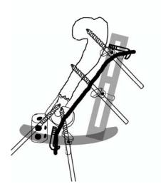
**8.** Connect a malleable stainless steel bar at its extremities to the hooks, in order to complete the strut contruct, and tighten the nuts on the hooks to firmly clamp the bar.
