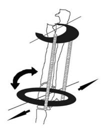
**7.** Perform the requested adjustment of torsional deformities by rotating the rings (you may require hemisphere nuts and washers for this procedure)
