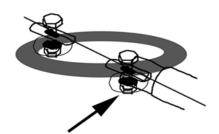
**15.** When you are satisfied with the wire's tension, tighten the nut on the near side of the ring
