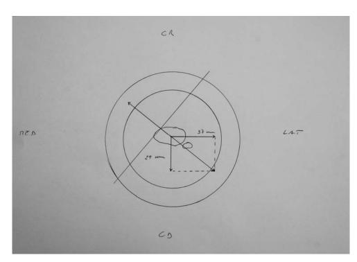
**5.** Draw the hinges' position on the ring using the registered data.
