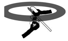
**5.** Stabilize the clamp with a wrench, and tighten the nut on the opposite side
