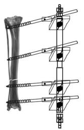
**10.** If you need to have inclined pins due to the fracture features, it's possible to use all the clamps with extensions, in order to hold them at the required angle
