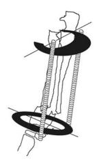
4. Connect the rings by means of threaded rods
