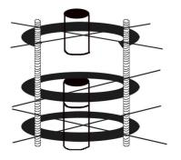
**6.** To start with bone transport: connect the middle ring to the bone, and perform an osteotomy distal to it, to obtain a bone cylinder for transport
