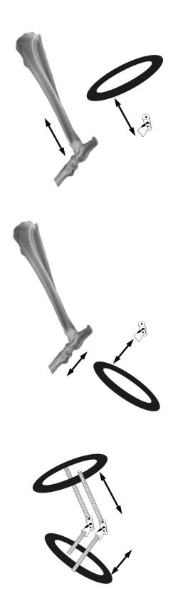
**1**. Once the appropriate procedure on the tarsal joint has been performed, measure the distance from the distal third of the tibia to the center of the tarsus. This will be the distance between the proximal ring and the hinge.
