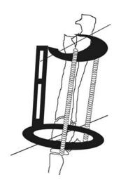
**9.** Up to this point, the circular and hybrid constructs are identical. If you want to set a hybrid contruct up,connect a rail to the distal ring, on the cranio-medial side of the radius
