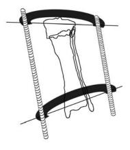
**3.** Connect the half rings with threaded bars and hemispherical nuts and washers
