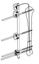
**9.** Bend the IM pin and connect it to the carbon bar by means of a clamp with a hook.
