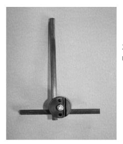
**3.** Connect the two bars tightening the double clamp by means of a M3 screw, in order to form a T frame.
