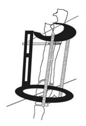
**10.** Insert a threaded pin in the radius, connecting it to the proxi-mal slot
