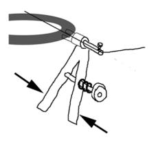
**11.** Tension the K wire pushing on the tensioner's handles
