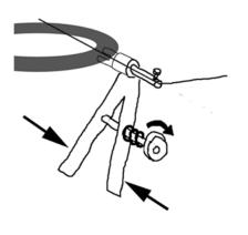
**12.** Lock the tensioner by tightening the locking nut on the side while maintaining the pressure on the handles
