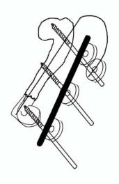
**6.** Complete the stabilization, and then connect the intramedullary pin with the proximal pin. In most cases, a single connecting bar is strong enough.
