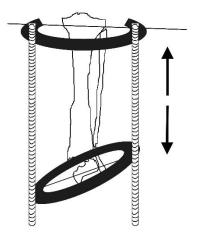
**5.** Distract the fracture by lengthening the threaded bars. Use two bars for standard distraction, three bars if the tension makes the fragment to incline
